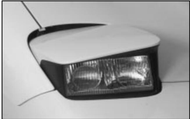
The headlamp doors are designed to open when you turn the headlamps on, and close when you turn the headlamps and parking lamps off. If you turn the headlamps on, then turn back to the parking lamps setting, the headlamp doors will stay open.
