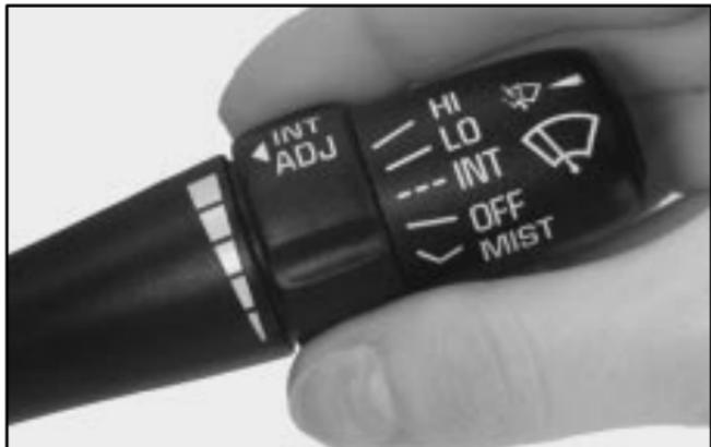
You can control the windshield wipers by moving the lever with the wiper symbol on it. This lever is located on the right side of the steering column.
