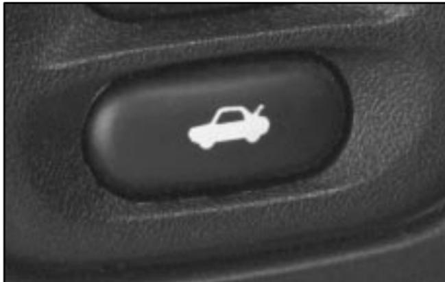
To use the hatch/trunk lid release on vehicles with an automatic transmission, your vehicle must be in PARK (P) or NEUTRAL (N). For manual transmissions, set the parking brake. See "Parking Brake" in the Index.
