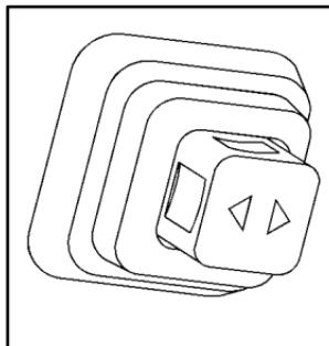
To operate the telescopic steering wheel, push the switch forward and the wheel will move away from you. Pull the switch rearward and the wheel will move toward you.
