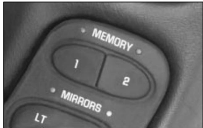
MEMORY can store and recall the settings for the driver's seat position, the outside rearview mirror positions, telescopic steering wheel (if equipped), radio presets, tone, volume, playback mode (AM/FM, tape or CD), last displayed station, compact disc position and tape direction and the last climate control setting.
