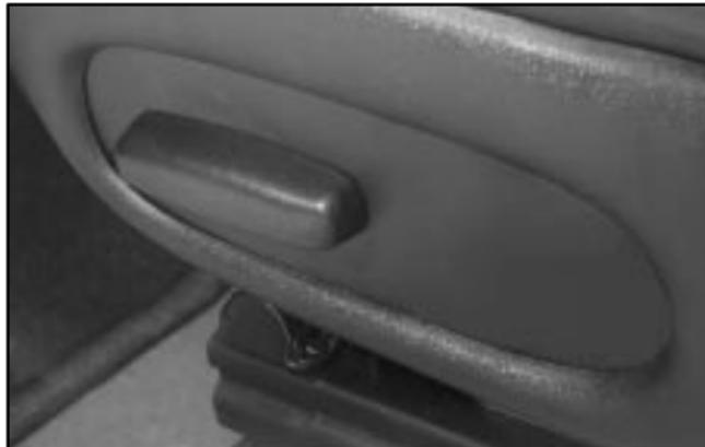
The control for the power seats is located on the outboard side of each seat, near the base.
