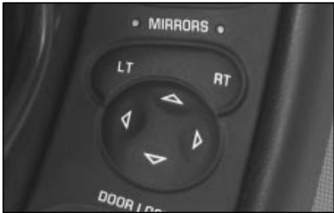
The electric mirror control is on the driver's door. It controls the driver's and passenger's mirrors. To adjust either mirror, press the LT (left) or RT (right) button to select the mirror, then press the arrows to adjust the direction of the mirror. The mirror will stay selected for 20 seconds after the last adjustment. An indicator light will come on above the mirror that you select.
