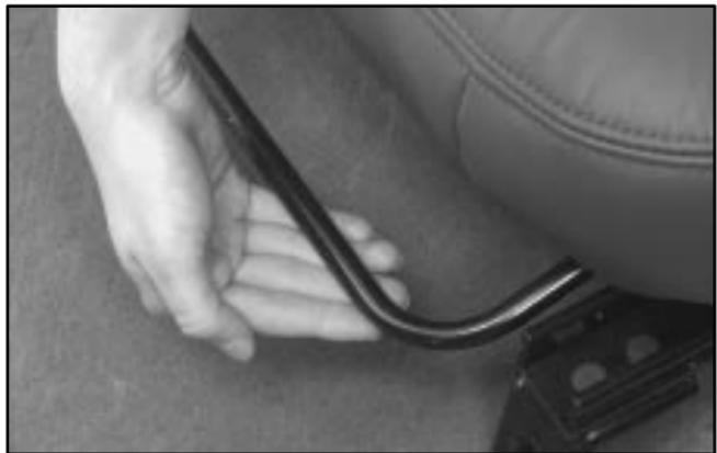
To move a manual seat, pull up on the lever located in front of the seat to unlock it. Slide the seat to where you want it. Then release the lever and try to move the seat with your body to make sure the seat is locked into place.
