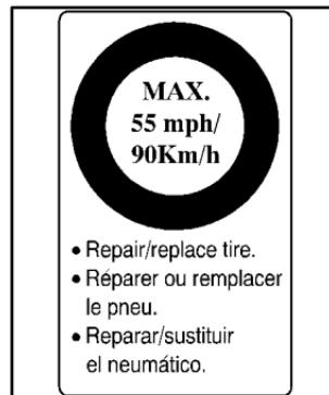
The maximum speed label reminds you to drive cautiously and not to exceed 55 mph (90 km/h) until you have the damaged tire inspected and repaired.
