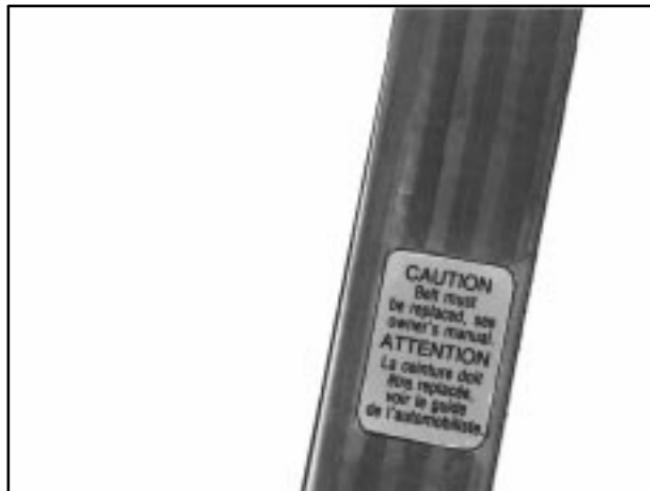
If you ever see a label on the driver's safety belt that says to replace the belt, be sure to do so. Then the new belt will be there to help protect you in a collision. You would see this label on the belt near the latch plate.
