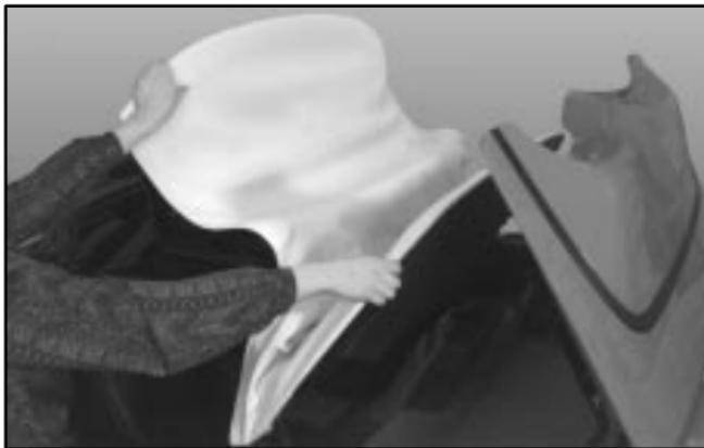
4. Lift the rear edge (B) of the convertible top to its full-up position by first raising the front edge (A).
