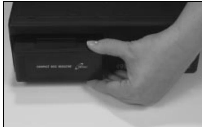
Once you have loaded the discs in the magazine, slide open the door of the compact disc (CD) changer. Push the magazine into the changer in the direction of the arrow marked on top of the magazine.
