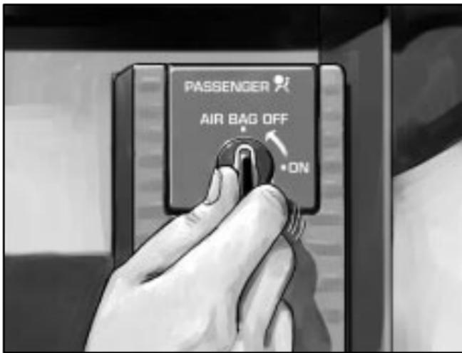
To turn off the passenger's air bag, insert your ignition key into the switch, push in, and move the switch to AIR BAG OFF.
