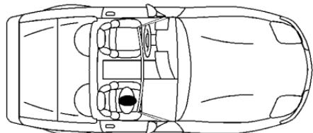
Your vehicle has a passenger air bag. There's an air bag off switch in the glove box you can use to turn off the passenger's air bag when you want to secure a rear-facing child restraint at the passenger's position. See "Air Bag Off Switch" in the Index for more on this, including important safety information.
