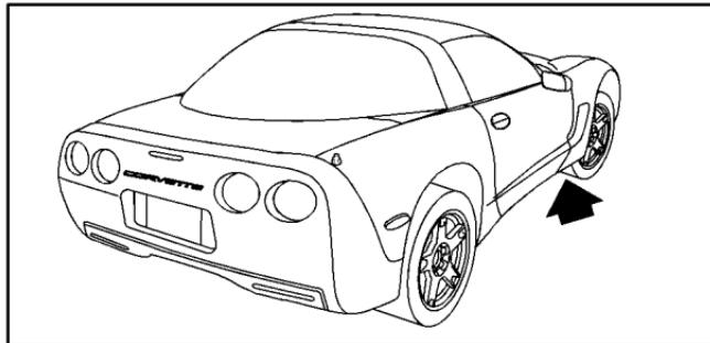
The front lifting point can be accessed from either the driver's or passenger's side of the vehicle, behind the front tires.
