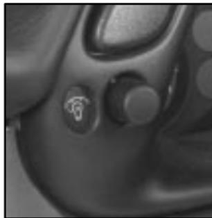
This knob controls the brightness of the instrument panel lights when the headlamps or parking lamps are on.
