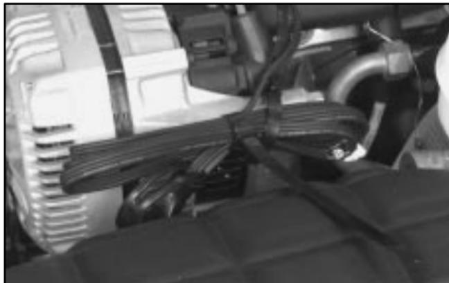
The engine coolant heater is located on the driver's side of the engine under the manifold.
