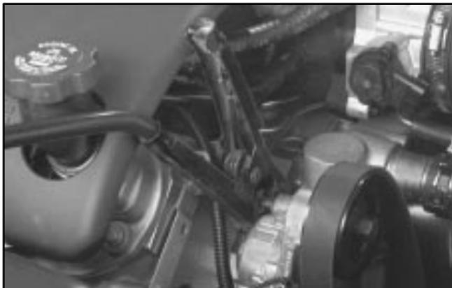
9. The other end of the negative (-) cable doesn't go to the dead battery. It goes to a heavy, unpainted metal part on the engine of the vehicle with the dead battery. Attach the cable at least 18 inches (46 cm) away from the dead battery, but not near engine parts that move. The electrical connection is just as good there, but the chance of sparks getting back to the battery is much less.
