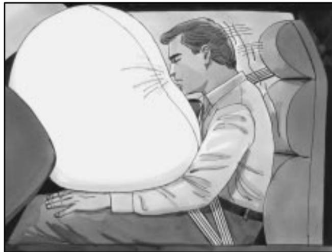
The passenger's air bag is in the instrument panel on the passenger's side.
