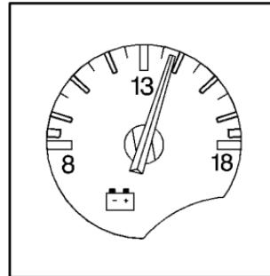
When the key is in ON with the engine not running, the voltmeter shows the voltage output of your battery. When the engine is running, it shows the voltage output of the charging system.
