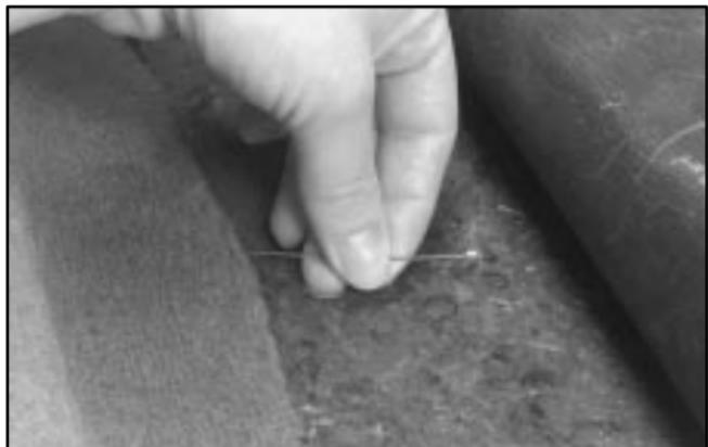
The cable is located underneath the carpeting behind the driver's and passenger's seats, in the center of the vehicle. When using the manual release, you must first open the doors to prevent damage to the seals. To access the cable, lift and pull back the carpeting. Then pull the cable to release the storage compartment lid if needed.
