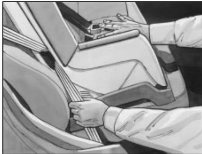
To remove the child restraint, just unbuckle the vehicle's safety belt and let it go back all the way. The safety belt will move freely again and be ready to work for an adult or larger child passenger.
