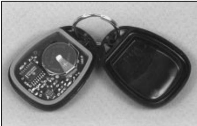
1. Insert a coin into the slot on the back of the transmitter and gently pry apart the front and back.
