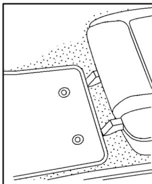
To remove the floor mats, pull up on the rear of the mat to disconnect from the locator hooks.
