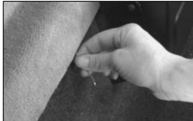
Pull the cable straight down to release the trunk lid.
