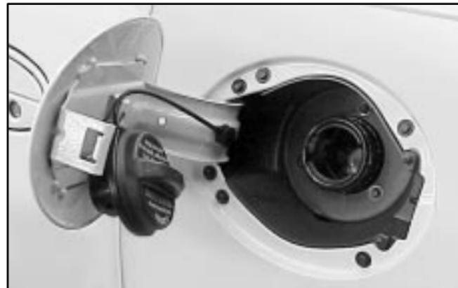
While refueling, rest the tether across the tab on the fuel filler door to prevent damage to your vehicle's finish.
