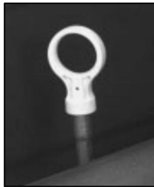
The engine oil dipstick handle is a yellow ring located near the coolant surge tank. See “Engine Compartment Overview” in the Index for more information on location.
