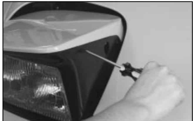
2. Remove the screws using a screwdriver on each side of the headlamp bezel.
