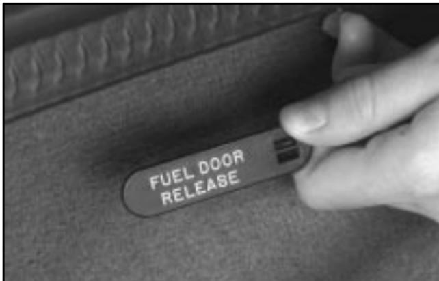
If your fuel filler door release won't operate, there is a manual release tab. The tab is located against the upper trim on the driver's side in the rear compartment. Pull the tab to manually release the fuel filler door.
