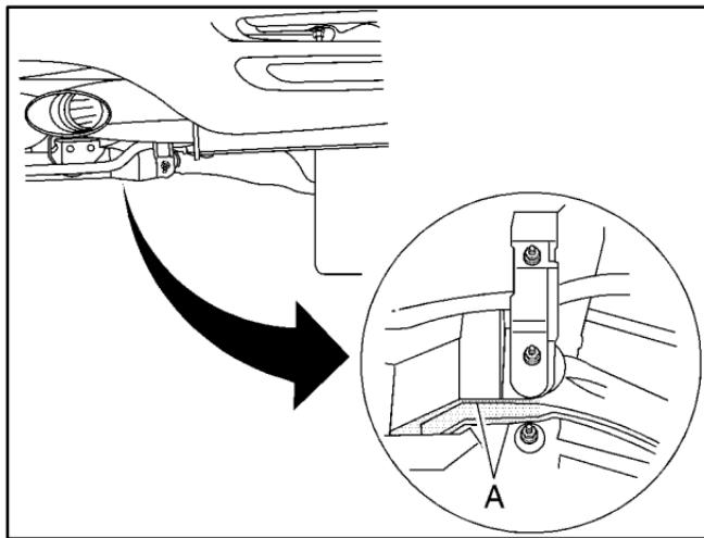
1. Locate the lifting point to jack your vehicle according to the illustration shown.
