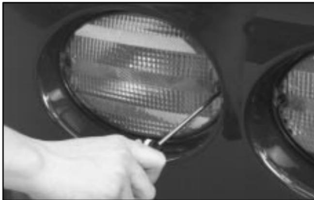
1. Remove the screws using a Torx® screwdriver.
