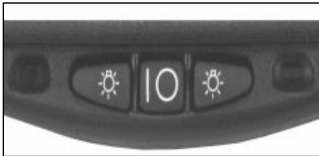
The mirror includes two map lamps and an automatic dimming function.
