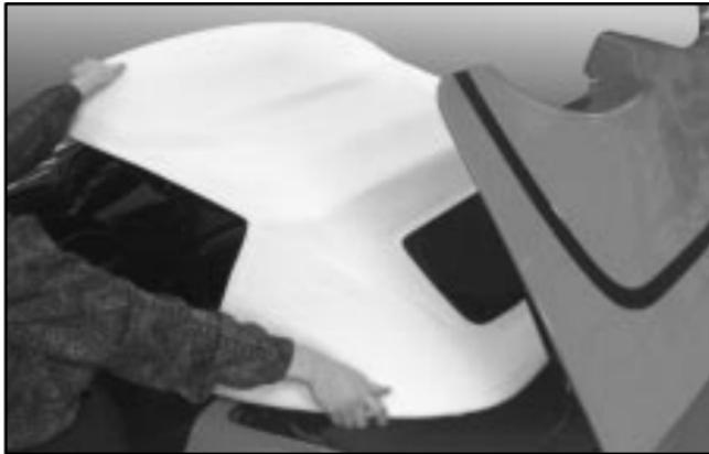
6. Push forward on the front edge (A) of the convertible top to allow the rear edge (B) of the convertible top to be moved to its full-down position.
