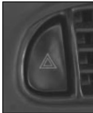
Press this button to make your front and rear turn signal lamps flash on and off.
