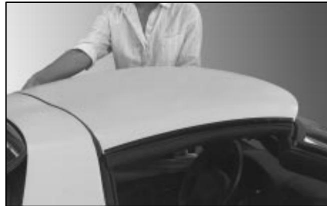
7. To unlock the rear of the roof panel, press the latch release button with your thumb and pull down the latch lever with your fingers.
