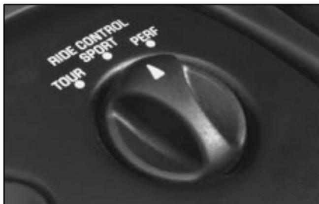
This switch is located on the center console. Turn it to select the suspension of your choice.
