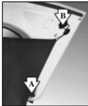
1. Hook the elastic loops on the front corners (A) of the shade to the T-nuts located on the front corners of the rear hatch frame.
