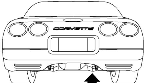
The rear lifting point can be accessed from the rear of the vehicle, on either the driver's or passenger's side.
