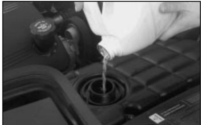
3. Then fill the coolant surge tank with the proper mixture, to the FULL COLD mark on the coolant surge tank.
