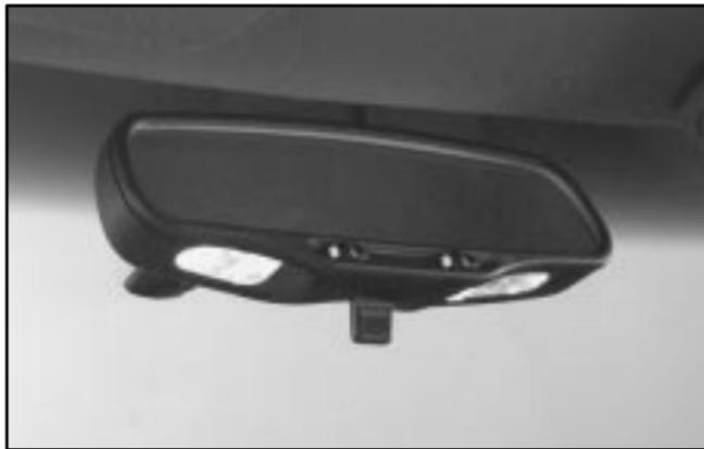
Your inside rearview mirror includes two reading lamps. The lamps will go on when a door is opened. When the doors are closed, each lamp can be turned on individually by pressing the switch (each lamp has its own switch).
