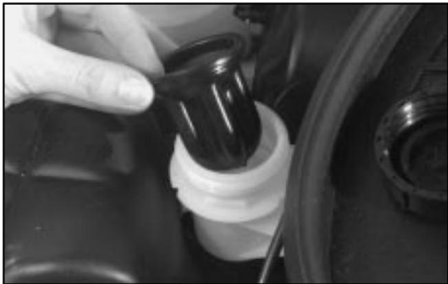
Fluid should be added if the fluid level is below the step on the inside of the reservoir. There are additional instructions on the reservoir cap. Put the rubber seal and cap back on. See "Engine Compartment Overview" in the Index for more information on location.
