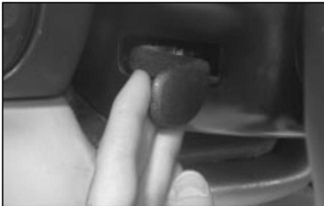
The lever is located on the left side of the steering column. To tilt the wheel, hold the steering wheel and pull the lever toward you. Move the steering wheel to a comfortable level, then release the lever to lock the steering wheel into place.
