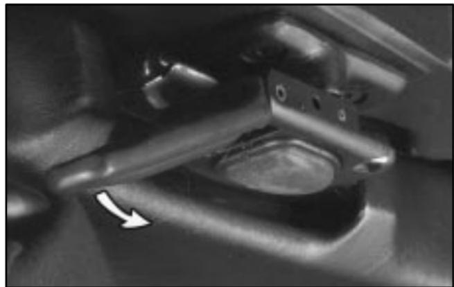
6. To unlock the front of the roof panel, pull down each of the front handles. Grasp the handles with your fingers and pull each toward you. Complete a  $180^{\circ}$  turn toward the center of the vehicle. Then push up on each of the handles.
