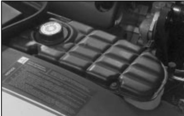
The coolant surge tank is located in the engine compartment behind the passenger's side headlamp. See "Engine Compartment Overview" in the Index for more information on location.
