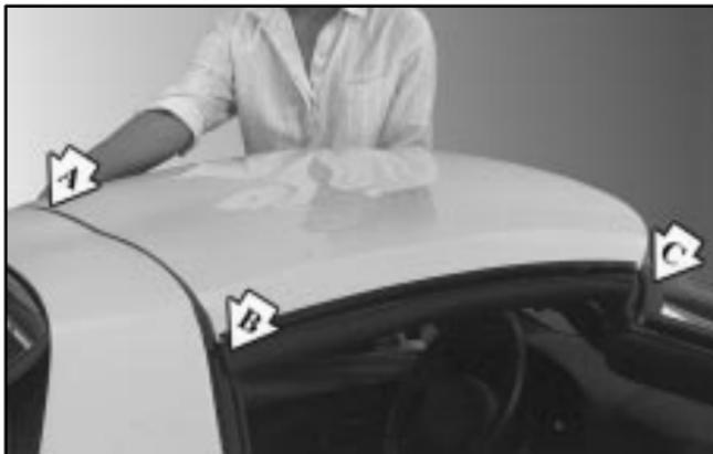
5. Position the rear edge of the roof panel to the weatherstrip on the back of the roof opening (A). Then align the pins at the rear of the roof panel weatherstrip with the receiving cup in the body weatherstrip (B). Gently lower the front edge of the roof panel to the front of the body opening (C).
