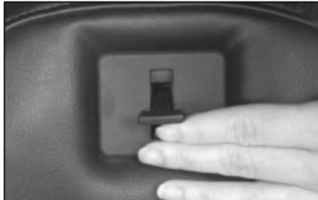
Both seatbacks fold forward to give you access to the rear area. To fold a seatback forward, lift this latch, which is located on top of the backside of the seat, and pull the seatback forward. The seatback will lock down in this position. To unlock, lift up on the latch and push the seatback rearward. When you return the seatback to its original position, make sure the seatback is locked in place.
