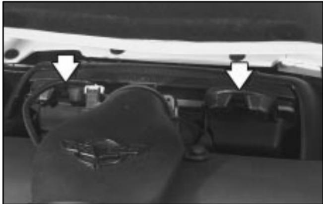
1. Pull up on the clips on each side to release the assembly.
