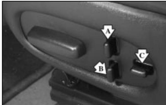
If your vehicle is equipped with a sport seat, there are three other controls that help you change the shape of the seat in addition to the power seat control. There are two lumbar supports for the middle (A) and lower (B) back. There's also a side bolster control (C) that adjusts the sides of the seat around you to give you more lateral support.
