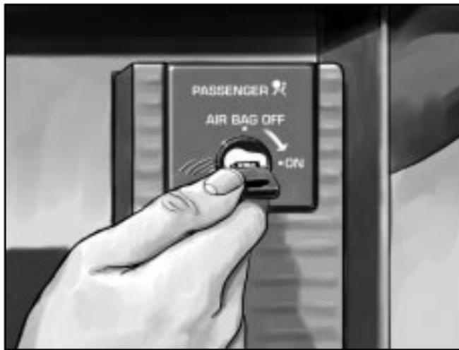
To turn the passenger's air bag on again, insert your ignition key into the switch, push in, and move the switch to the ON position.
