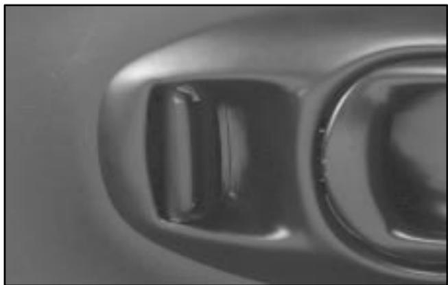
To lock the door from the inside, move the lever located on the door forward. To unlock it, move the lever on the door rearward.
