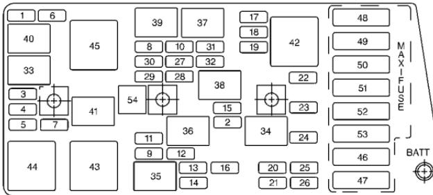
There is one fuse block in the engine compartment located on the passenger's side of the vehicle in front of the battery.
