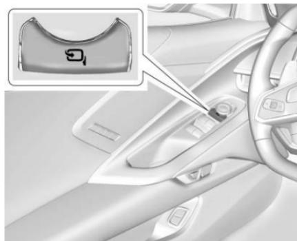
If equipped, press
