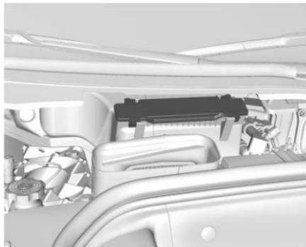
3. Press two push tabs on the top and on the bottom of the cabin air filter cover and remove the cover.
