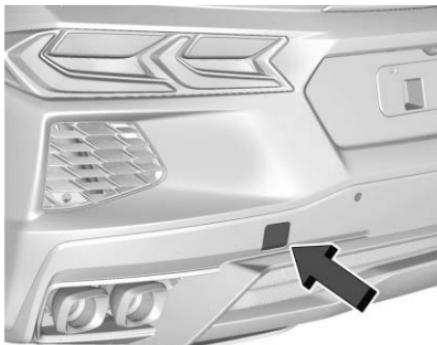
Carefully open the cover by using the small notch that conceals the rear tow eye socket.
