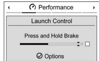
1. Using the Driver Information Center buttons on the right side of the steering wheel, navigate to the performance menu. See *Instrument Cluster* ▷ 81.
