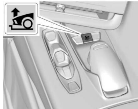
To use the Front Lift System, press the button on the center console to raise or lower the vehicle. This feature can be operated at speeds up to 38 km/h (24 mph) when the engine is running. The system functions based on the vehicle's state or operating mode:
