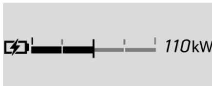
The electric power indicator gauge is in the bottom of the display to the right of the speedometer, and is only shown in the Shuttle mode.
