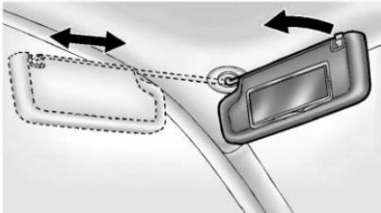
Pull the sun visor down to block glare. Detach the sun visor from the center mount to pivot to the side window and, if equipped, extend along the rod.
