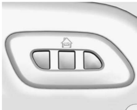
If equipped, these buttons are in the sunshade. This system can replace up to three remote control transmitters used to activate devices such as garage door openers, security
