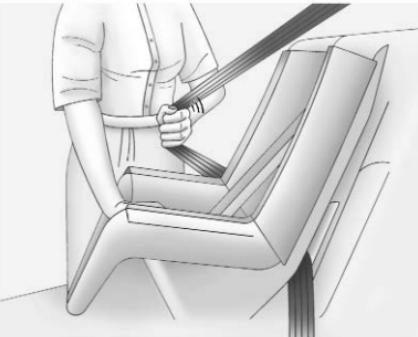
6. Pull the shoulder belt all the way out of the retractor to set the lock. When the retractor lock is set, the belt can be tightened but not pulled out of the retractor.
