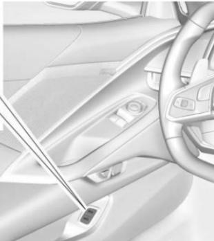
1. With the transmission in P (Park), press
