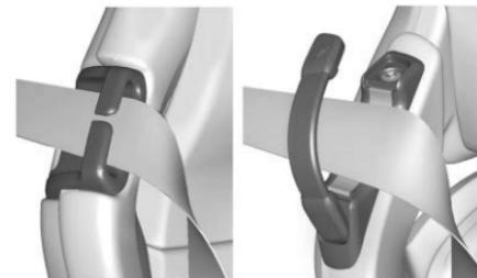
2. Be sure that the shoulder belt is routed through the seat belt guide. See *Lap-Shoulder Belt* ▷ 48 for proper belt routing.
