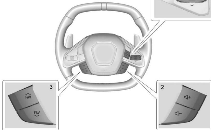
If equipped, some audio controls can be adjusted at the steering wheel.
