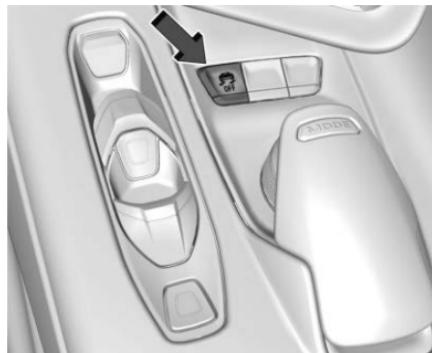
The Traction Control System/StabiliTrak/Electronic Stability Control button is on the center console.
