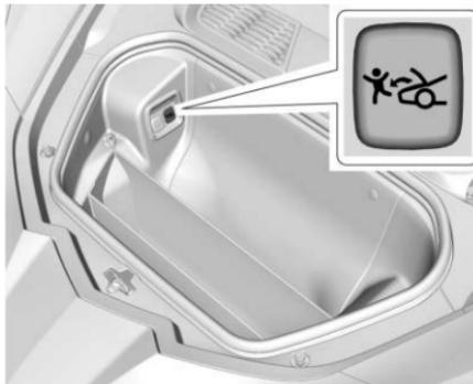
The underhood compartment may be equipped with a glow-in-the-dark emergency hood release button. This button will glow following exposure to light. Press the button to open the hood from inside the underhood compartment.
