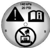
2. When the cooling system, including the coolant surge tank pressure cap and engine, is no longer hot, remove the pressure cap.
