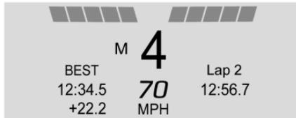
**Track:** Displays the vehicle speed, gear position, shift lights, and current/best lap times. This includes Gain/Loss of Current Lap compared to Best Lap.
