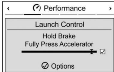
6. Return to the landing page of Launch Control. Firmly press and hold the brake pedal to activate Launch Control.
