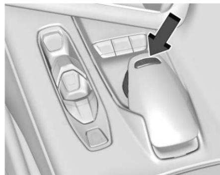
To activate My Mode, Weather, Tour, Sport and Track mode, turn the DMC knob on the center console to make a mode selection. When a mode is selected, an indicator will come on in the instrument cluster and stay on. See "E-Ray – EV Drive Mode Activation" later on in this section for details on activating EV drive modes.
