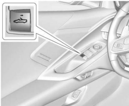
6. Pull and hold
