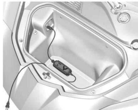
Some vehicles have a battery maintainer package. Follow the instructions provided with the battery maintainer package to keep the battery charged when the vehicle is not in use. Plug the battery maintainer into the underhood accessory power outlet only. For ZR1 models, use clips to connect to the battery directly.
