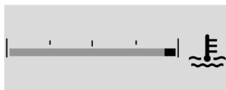
This gauge shows the engine coolant temperature.
