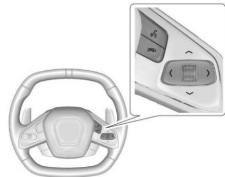
Press < or > to access the cluster applications. Use the thumbwheel to scroll ▲ or ▼ through the list of available features. Press the thumbwheel to select. Not all applications will be available on all vehicles.
