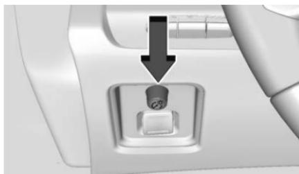
This feature adjusts the brightness of all illuminated controls. The knob for this feature is to the side of the steering wheel closer to the driver door.
