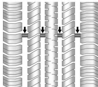
Treadwear indicators are one way to tell when it is time for new tires. Treadwear indicators appear when the tires have only 1.6 mm (1/16 in) or less of tread remaining. See *Tire Inspection* ▷ 316 and *Tire Rotation* ▷ 316.
