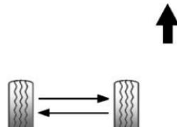
Use this rotation pattern if the vehicle has different size tires on the front and rear.
