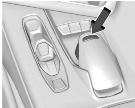
3. Turn the DMC knob. The selection menu displays on the instrument cluster with the available EV drive modes. The availability of an EV mode depends on various factors. See "EV Drive Mode Attributes" later on in this section.
