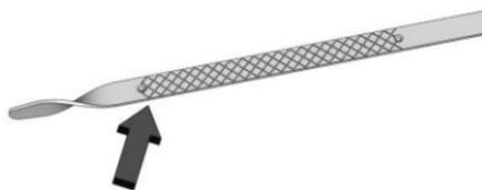
If the oil is below the cross-hatched area at the tip of the dipstick, add 1 L (1 qt) of the recommended oil through the oil fill cap opening in the oil tank fill tube and then recheck the level. See "Selecting the Right Engine Oil" later in this section for the type of oil to use. For engine oil crankcase capacity, see *Capacities and Specifications* ▷ 348.
