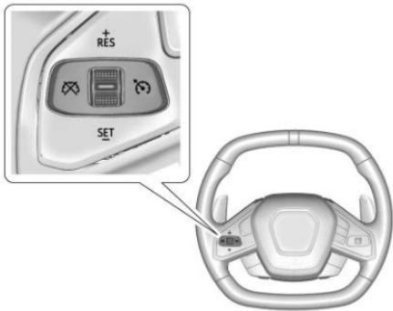
**Cruise:** Press to turn cruise control on or off. A white cruise control indicator light comes on in the instrument cluster when cruise is turned on.
