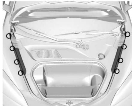
1. Release the four clips for the left and right outer covers.
