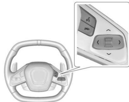
**< or >** : Press to move left or right between the interactive display zones in the cluster. Press the thumbwheel to select.
