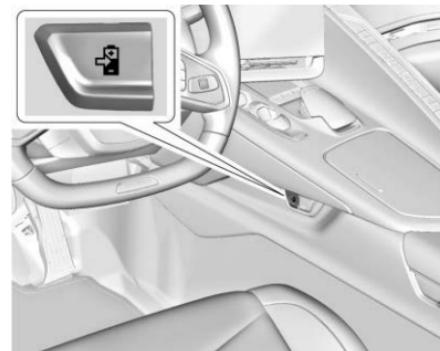
Press the Charge+ button on the driver side of the center console. When the Charge+ feature is active, the hybrid battery charging light displays on the DIC. See *Hybrid Battery Charging Light (Charge+)* ▷ 87. Also, a small pop-up window will also appear showing the exact SOC and electric power input/output. The Hybrid Battery Gauge shows the increasing SOC filling into the blue zone. See *Power Indicator Gauge* ▷ 87.
