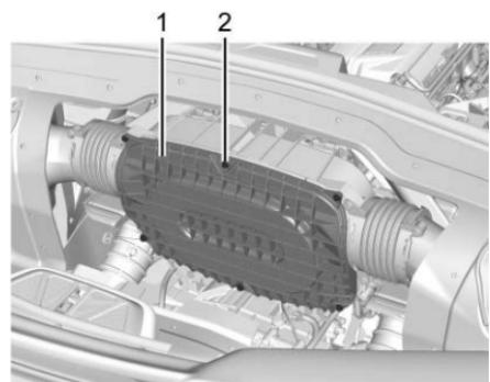
6. Remove the air cleaner cover screws (2) and cover (1).
