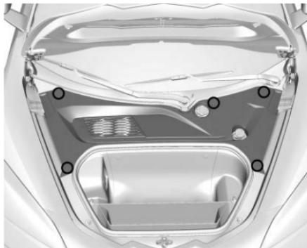
2. Release the five clips and remove the outer cover.
