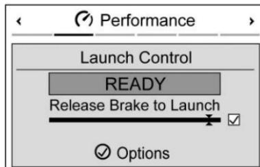
7. Fully press the accelerator. Release the brake pedal to launch the vehicle.
