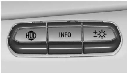
The HUD control is to the left of the steering wheel on the instrument panel.
