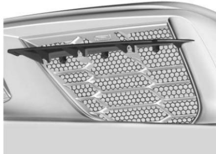
For vehicles with the optional Grille Screen Guards (VWE), remove them for track events when the ambient temperature reaches 32° C (90° F) or higher. See your dealer for complete procedure.
