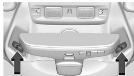
If equipped, the reading lamps are in the overhead console. The lamps go on when any door is opened,
