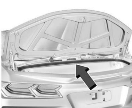
Use the pull cup to lower the hatch if needed, then drop into the latch or push on the outside of the panel until the power latch feature activates. The hatch/trunk will close the rest of the way and latch automatically.
