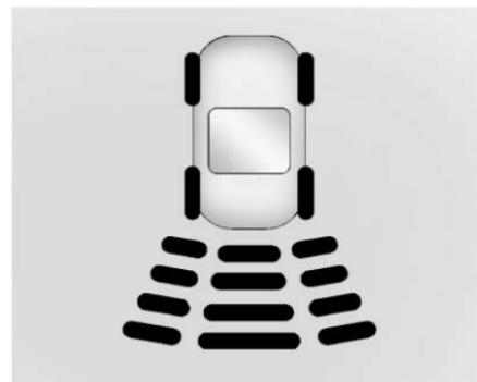
The instrument cluster may have a Park Assist display with bars that show "distance to object" and object location information for RPA. As the object gets closer, more bars light up and the bars change color from yellow to amber to red.
