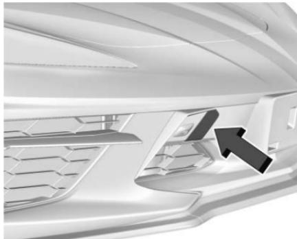
Carefully open the cover by using the small notch that conceals the front tow eye socket.
