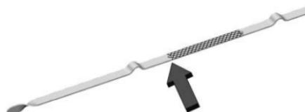
If the oil is below the cross-hatched area at the tip of the dipstick, add 1 L (1 qt) of the recommended oil through the oil fill cap opening in the oil tank fill tube and then recheck the level. See "Selecting the Right Engine Oil" later in this section for the type of oil to use. For engine oil crankcase capacity, see *Capacities and Specifications* ▷ 348.
