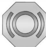
The brake master cylinder reservoir is filled with GM approved DOT 4 brake fluid as indicated on the reservoir cap. See *Underhood Compartment Overview* ▷ 247 for the location of the reservoir.
