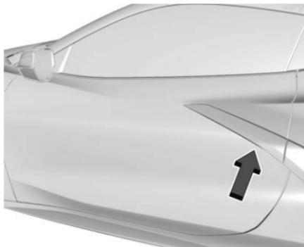
For Keyless Access, hold the remote key within 1 m (3 ft) of the door handle. Grip and press the door handle touchpad. See *Remote Key Operation* ▷ 8. This feature can
