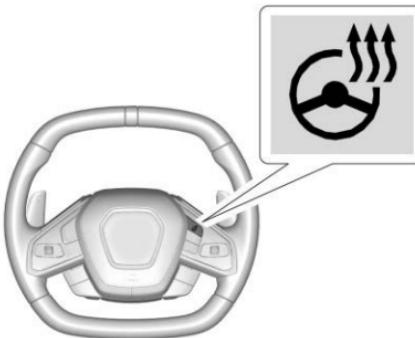
➊ If equipped, press to turn the heated steering wheel on or off. A light next to the button displays when the feature is turned on. The steering wheel takes about three minutes to be fully heated.
