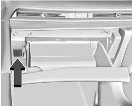
The PDR records video, audio, and vehicle data. The forward facing video and cabin audio are captured by a camera and microphone located behind the rear view mirror. The PDR video and data is stored on a removable SD card located in the SD card reader in the glove box. The video (MP4) can be played back in the vehicle or the SD card can be removed and played on a PC or a mobile device, or the file can be viewed and analyzed within Toolbox. See Toolbox later in this section.
