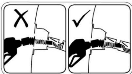
The capless system has two internal flapper doors. To prevent fuel spray, insert the nozzle fully to ensure both doors are open before refueling.
