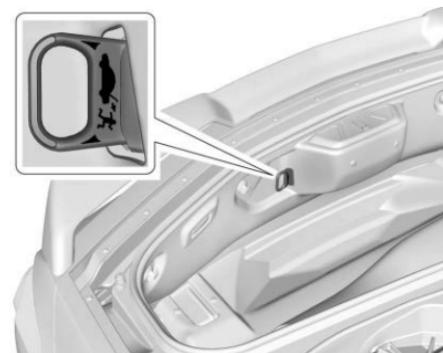
There is a glow-in-the-dark emergency hatch/trunk release handle on the inside back wall of the storage compartment. This handle will
