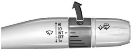
**INT:** Move the lever up to INT for intermittent wipes, then turn the
