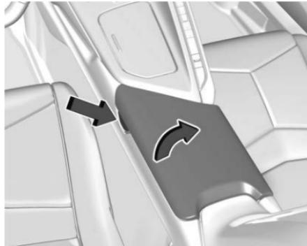
To open, press the button on the driver side.
