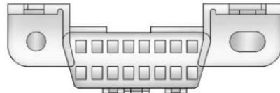
The DLC is under the instrument panel to the left of the steering wheel. Connecting devices that are not used to perform an Emissions Inspection/Maintenance test or to service the vehicle may affect vehicle operation. See *Add-On Electrical Equipment* ▷ 243. See your dealer if assistance is needed.
