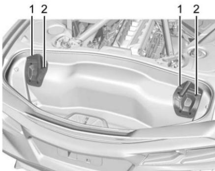
2. Remove the four lift off bracket bolts (2) to remove the brackets (1).
