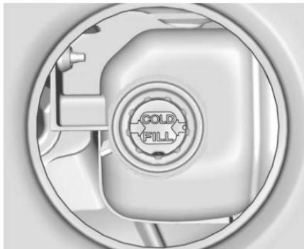
4. Fill the coolant surge tank with the proper mixture until the level inside stabilizes at the COLD FILL indicator in the surge tank.
