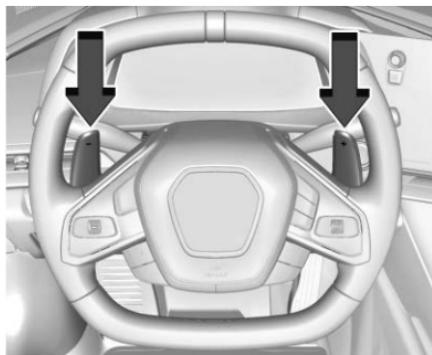
With the transmission in D (Drive), press the M (Manual Mode) switch on the center console to enter Manual Mode. Use the paddles on the steering wheel to manually upshift or downshift the transmission. The right + (plus) paddle upshifts, and the left - (minus) paddle downshifts.
