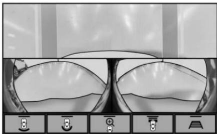
If equipped, a view of the area in front of the vehicle displays in the infotainment display. The display shows a front, top down view at the top and left and right front camera images on the bottom.
