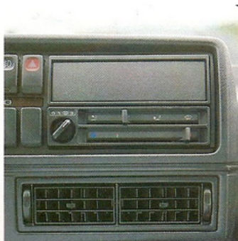
4 buses centrales de ventilation
